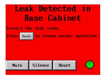
This button takes the user back to the Main screen after the Leak Detected alarm has been Silenced or Reset.
