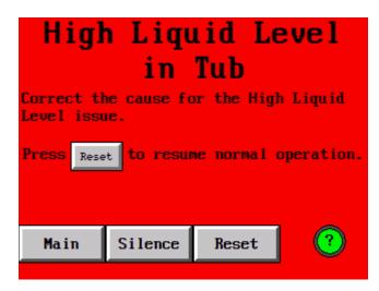
This button takes the user back to the Main screen after the High Liquid Level in Tub alarm has been Silenced or Reset.
