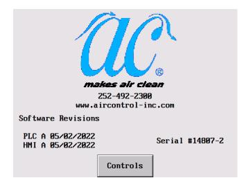
This screen is the first screen that comes up on the touchscreen controller when the hood is powered up. It lists the benches serial number, as well as the software revisions of the operating software.
